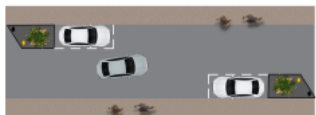
Chicane parking arrangement with build outs
